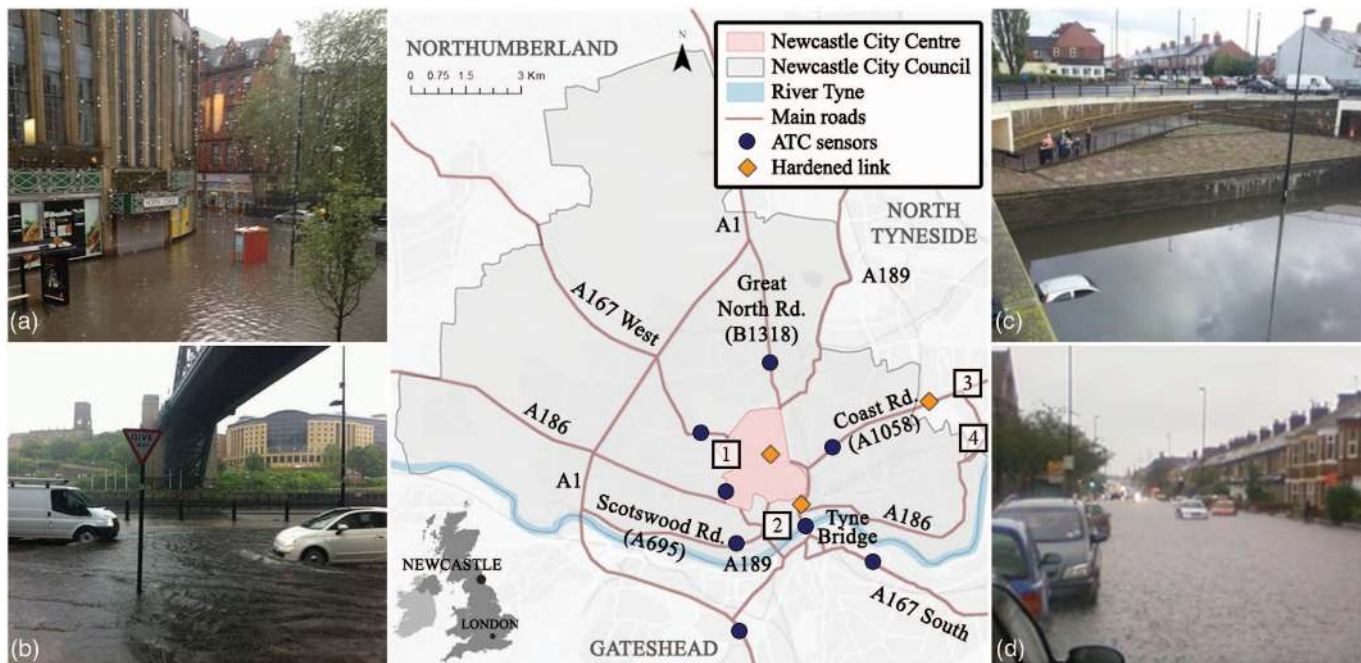
Fig. 1. (Color) Newcastle map with photos taken during June 28, 2012; a bow wave shows that vehicles continue to move, albeit slowly, at (b) the Quayside and (d) Chillingham Road, but not in images (a) and (c) where the flood water is too deep (photos courtesy of Newcastle University; map source: Esri, DigitalGlobe, GeoEye, Earthstar Geographics, CNES/Airbus, DS, USDA, USGS, AEX, Getmapping, Aerogrid, IGN, IGP, swisstopo, and the GIS User Community)
