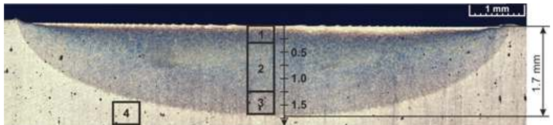
Figure 4: Microstructure of the surface layer at x50 magnification of experiment N°4.
