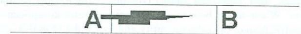
Fig. 3. Two special cases of operator error: (A) when mark is within defect, and (B) when mark is beyond defect.
