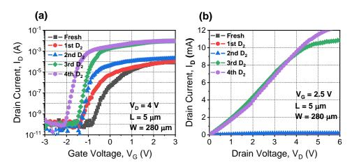
**Figure 3.** Measured (**a**)  $I_D$ - $V_G$  and (**b**)  $I_D$ - $V_D$  characteristics of the fabricated device after iterative deuterium annealing.
