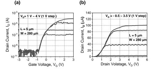
**Figure 2.** Measured (a)  $I_D$ - $V_G$  and (b)  $I_D$ - $V_D$  characteristics of fabricated TV device before deuterium annealing.
