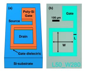
**Figure 1.** (a) Schematic and (b) optical microscope image of test vehicle on which silicon substrate is fabricated.
