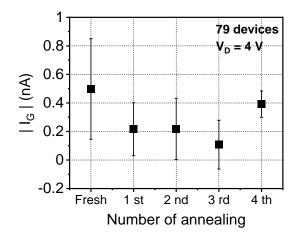
**Figure 5.** Extracted gate leakage ( $I_G$ ) after iterative HPD. The  $I_G$  was extracted at  $V_G = -3$  V.
