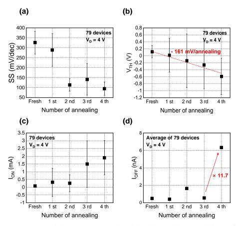
**Figure 4.** Extracted device parameters such as (a) SS, (b)  $V_{TH}$ , (c)  $I_{ON}$ , and (d)  $I_{OFF}$  after iterative HPD. The symbol and error bar indicate the average value and standard variation, respectively.  $I_{ON}$  and  $I_{OFF}$  were extracted at  $V_G = V_{TH} + 2 V$  and  $V_G = V_{TH} - 2 V$ , respectively.
