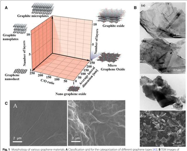
Fig. 1 Morphology of various graphene materials. A Classification grid for the categorization of different graphene types [43]. B TEM images of graphene nanoplates (1–5 nm), graphene nanoplates (5–20 nm), micro-graphite, and SEM image of natural graphite (top to bottom) [50]. C SEM images of GO (a) and ERGO (b) [118]
