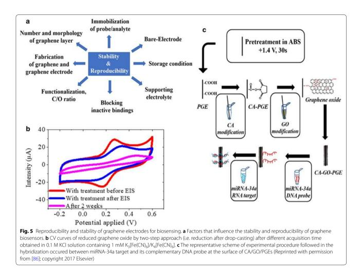
orientation of the biomolecules on the electrode surface, favouring efficient aptamer/analyte hybridization. Unlike adsorption-based methods, the charge transfer resistance continued to increase upon analyte hybridization due to a more negatively charged species on the surface of the electrode and repulsion of  $[Fe(CN)6]^{3-/4-}$  by the negatively charged phosphate backbone of the hybridized DNA probe [129]. This improved sensitivity for electrochemical analyte detection.
