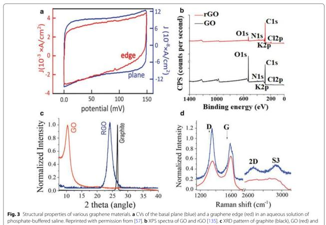
rGO (blue) [74]. d Raman spectra of GO (red) and rGO (blue) [74]. After reduction the intensity ratio between D and G (I(D)/I(G) increased
