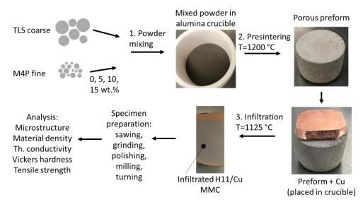
**Figure 2.** Preparation of H11/Cu MMCs, including the steps of powder mixing, presintering to obtain a porous preform and infiltration of the preform with molten copper.
