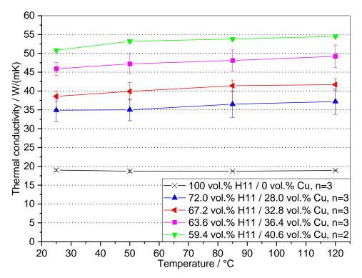
**Figure 7.** Thermal conductivity  $\lambda$  of the four manufactured H11/Cu composite materials and the sintered H11 tool steel as a function of temperature.
