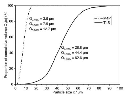
**Figure 1.** Powder particle size distribution (PSD) of the employed fine M4P H11 powder and the coarse TLS H11 powder.
