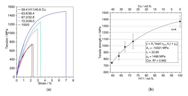
**Figure 9.** (a) Stress-strain curves and (b) tensile strength of the H11/Cu composite materials obtained by infiltration and the sintered H11 tool steel as a function of H11 content.
