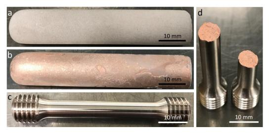
**Figure 3.** Stages in preparation and testing of the H11/Cu tensile testing specimens with (**a**) porous H11 preform, (**b**) copper infiltrated blank, (**c**) machined H11/Cu tensile specimen and (**d**) tensile specimens subsequent to tensile testing.
