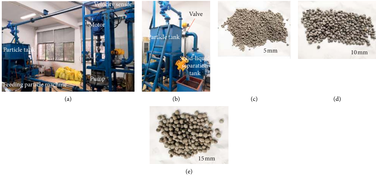
FIGURE 20: The experiment system and particles: (a) overall view of the test system, (b) side of the test system, (c) 5 mm particles, (d) 10 mm particles, and (e) 15 mm particles.
