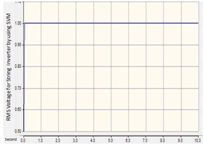
Figure 21. RMS-output of string inverter using SVM.
