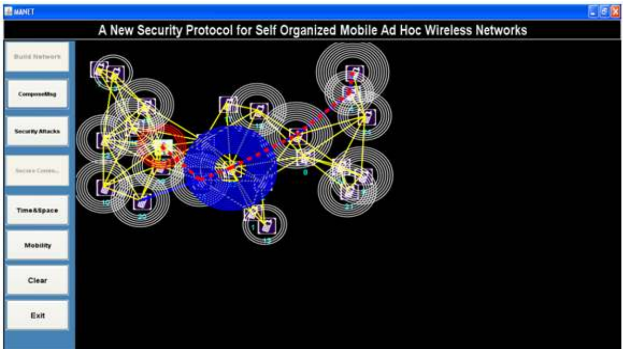
Figure 6: A snapshot of showing a Sybil attacker spoofing the identities of other nodes and forwarding data to destination as if the actual node is forwarding data
