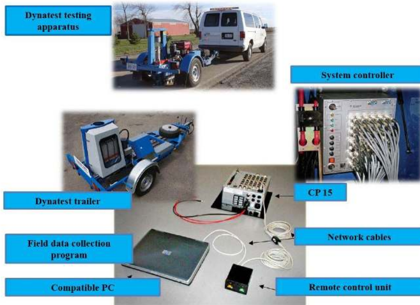
Fig. 5. General view of dynamic loading test apparatus Dynatest and its main components.
