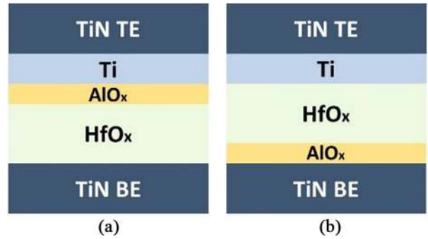
FIGURE 1. Schematic diagrams of RRAM devices with (a) TiN TE/Ti/AlO x /HfO x /TiN BE and (b) TiN TE/Ti/HfO x /AlO x /TiN BE stacked layers. And both HfO x and AlO x dielectric films were amorphous structure.
