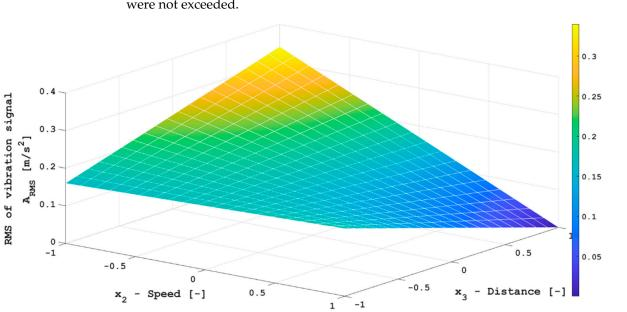
values obtained for the surface–paving stones exceeded the limit of vibrations to which a person can be exposed, which was equal to  $A_{RMS} = 0.8 \text{ m/s}^2$ . For other surfaces, the values were not exceeded.
