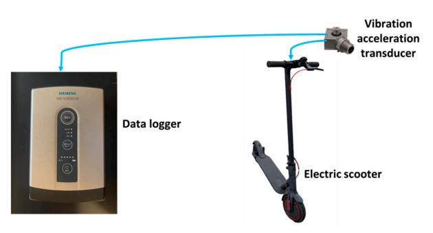
Figure 2. Diagram of the installation of the measuring sensor and the recording system.
