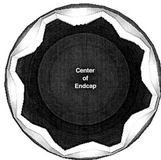
FIGURE 8 Cross-sectional view of projectile 0.80 ms after impact revealing circumferential buckling mode (scale factor = 20.0).
