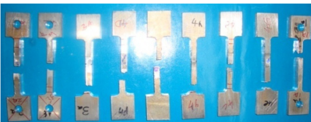
Figure 8: Photographic View of the sample of the tensile test specimen after tensile testing
