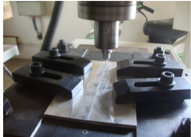
Figure 2: Initial Joint Configuration arrangement of AZ31B Mg Alloy flat plates in the Fixture along with the taper cylindrical pin profiled HSS tool
