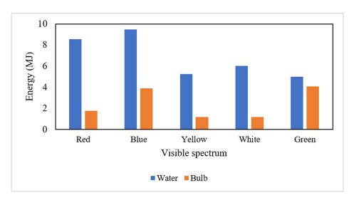
**Figure 6.** Energy inputs of water and light for growing attached microalgae on palm decanter cake at various visible spectra of irradiation.
