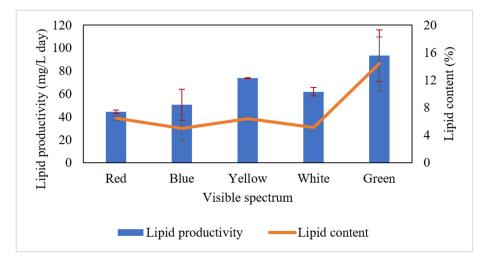
**Figure 2.** Lipid productivity and contents of attached microalgae growing on palm decanter cake at various visible spectra of irradiation.
