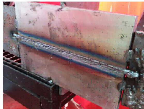
Fig.1. Welded sample of HY-80 steel after welding experiment
