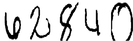
Fig. 4. Digits confused with under-segmented class by the second low-level verifier. This kind of 8 and 0 are sometimes misverified by the first verifier.
