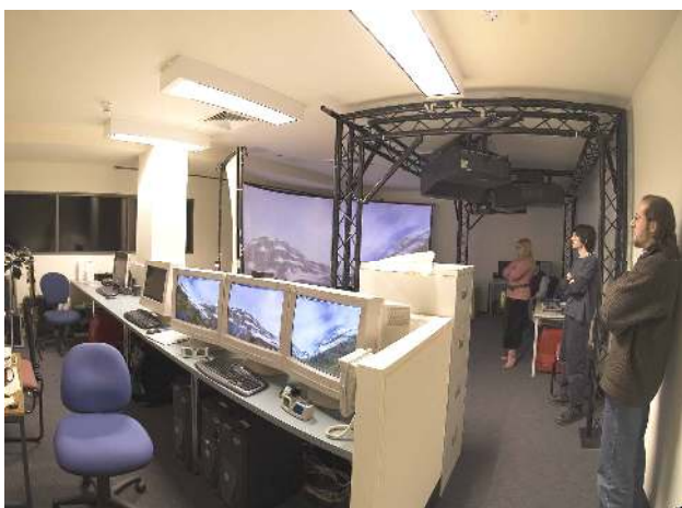
Fig. 12. VR Lab showing the three screen configuration in the foreground and VISOR in the background
