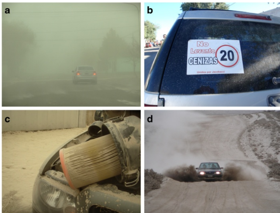
Fig. 12 Road conditions in Jacobacci a poor visibility In Jacobacci (11/7/2011); b 2WD car outside Jacobacci in ~50mm ash; c car air filter clogged with ash; d sticker on car window in Jacobacci advising drivers to restrict their speed to 20km/h in order to not "stir up the ash." (Photo credit: Ailen Rodriguez)
