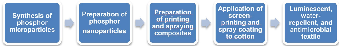
Fig. 1 Diagram demonstrates the preparation of multifunctional textiles via screen-printing and spray-coating technologies
