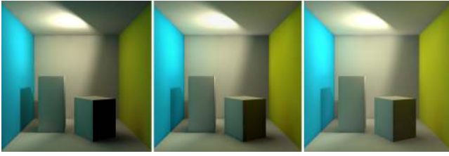
Figure 7: From left to right: One, two and three bounces of indirect illumination rendered at 1024 \times 1024 with 14.0, 7.5, and 5.5 fps respectively (using 1024 VPLs for the first bounce and 256 VPLs each for the second and third).
