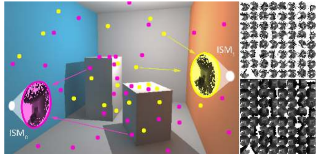
Figure 3: Global Illumination with imperfect shadow maps: The indirect light in this didactic scene is represented by two VPLs. Each VPL generates a shadow map using a point-based representation of the scene. Since coarse visibility information is sufficient, each VPL uses only a sparse subset of the points (encoded as colors) to generate an imperfect shadow map at real-time rates. The contribution of all VPLs is summed up yielding the final indirect illumination. Examples of imperfect shadow maps (bottom with and top without pull-push) are shown on the right; dark value signify small depth values and light values represent large depths.
