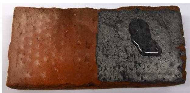
Supplementary Figure 4. Photograph demonstrating water permeation through a brick (~20 cm long) with and without VC-RGO coating. Brick without the graphitic coating rapidly absorbs water but it can stay on top of the VC-RGO coated part for many hours.
