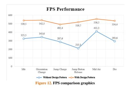
In **Figure 12**, information obtained from algorithms with a design pattern has a higher FPS and is more stable than algorithms that do not use design patterns. The weight of computing during JumpButtonRelease makes video game performance decrease for a moment, so players feel a lagging when characters move.
