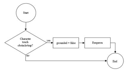
Figure 1. Functions inside OnTriggerEnter2D
