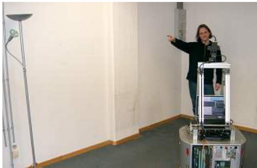
Figure 1: Interaction with our development system. Software components include: speech recognition, speech synthesis, person and gesture tracking, dialogue management and multimodal fusion of speech and gestures.
