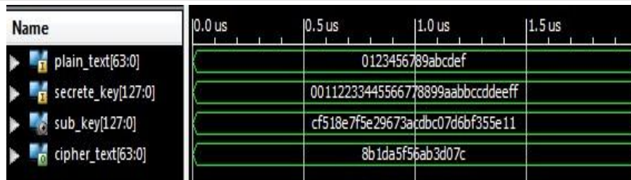
Figure 10. Simulation results of the MISTY1 module in encryption mode.
