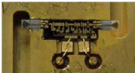
FIGURE 3. Example of a packaged 90–140 GHz MMIC amplifier utilizing E-plane probes with bond wire connections.
