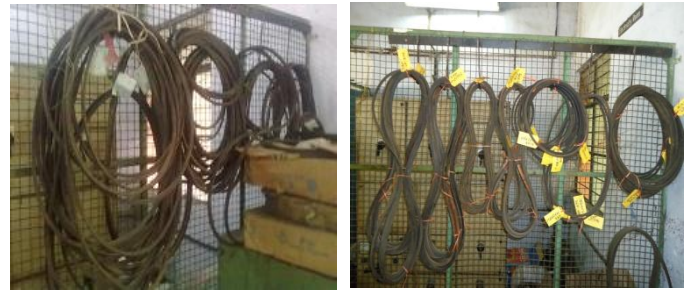
Fig. 7. Before & After pictures of 1S SEIRI (Sort)
