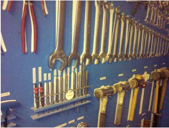
Fig. 2. The shadow board displaying all the equipment and tools at its right place.
