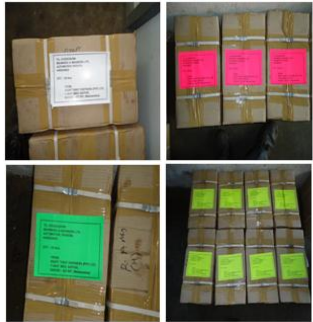
Fig. 10. Marking and Standardization of the Templates with different color codes. (each color code specifies a particular company/product which helps in minimizing the problem of dispatching the different product to other company).
