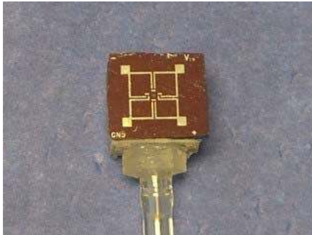
Figure 7. Pressure Sensor Mounted for Testing (left), and Experimental Data (right)
