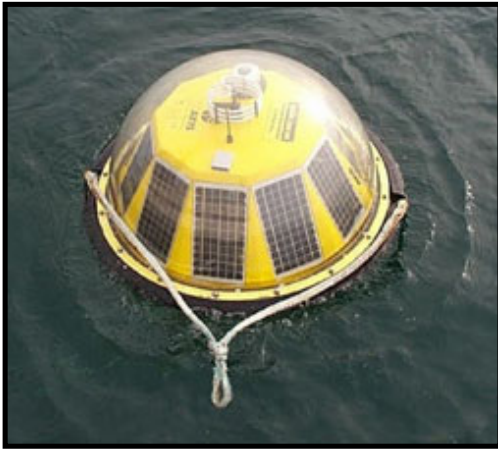
Fig. 1. NAVOCEANO's positioning and telemetry buoy
