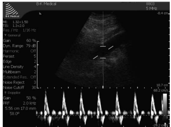
Fig. 9. Duplex interface on the Profocus scanner during data acquisition. All parameters listed to the left are also registered in the usecase produced in each data acquisition sequence.
