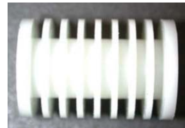
Fig. 15. Bobbin for the igniter transformer.
