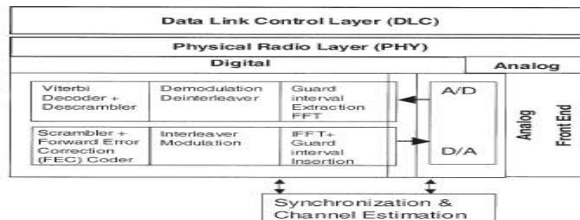
Figure 7 Block diagram of the physical layer of an IEEE 802.11a Transceiver
