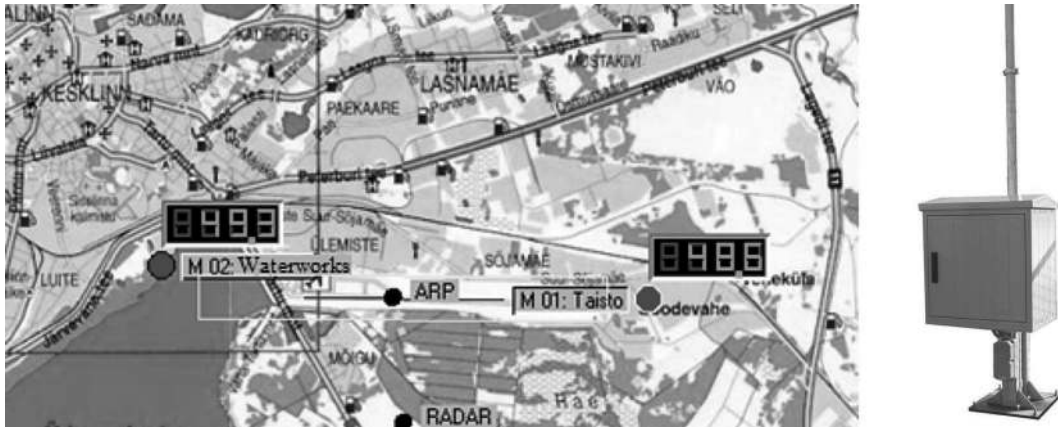
Fig. 1. Noise monitoring station (right) and their locations (left). (Keskküla 2012b)
