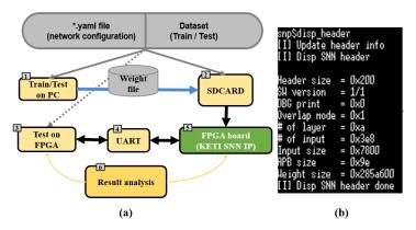
**Figure 5.** The data flow in the FPGA board. (**a**) Data pipeline for training and testing scenarios where \* represent the name of the .yaml file and numbers represent the order of the tasks in a sequence; (**b**) FPGA SNN environment with header and deployment arguments.
