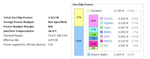
Figure 16. FPGA (xcku115-flvf1924-2-i) power utilization in dynamic mode (deploying DCSNNs).
