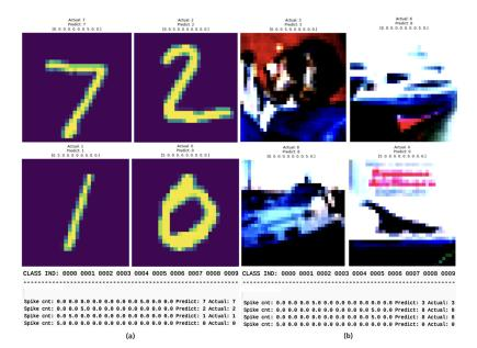
**Figure 6.** Spike-based data prediction on FPGA board. (**a**) Spike prediction on FPGA board (MNIST); (**b**) spike prediction on FPGA board (CIFAR10).
