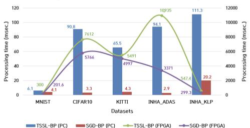
Processing times of TSSL-BP & SGD-BP on FPGA alongside PC
