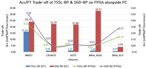
Figure 15. Comparison between trade-off metrics of TSSL-BP and SGD-BP on FPGA alongside PC.
