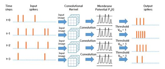
Figure 2. Schematic of deep convolutional spiking neural networks.
