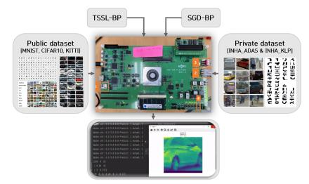
Figure 1. Implementation schematic of DCSNN using spike-based backpropagation on FPGA platform.
