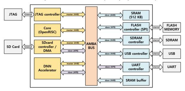
Figure 4. The overall block schematic of the FPGA board design.
