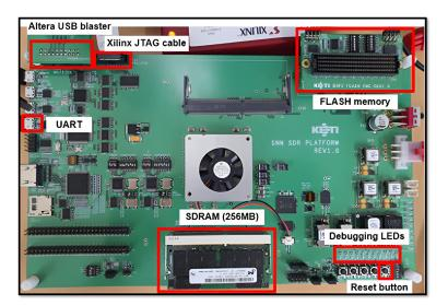
Figure 3. The external view of the on-chip FPGA spiking neural network processor.
