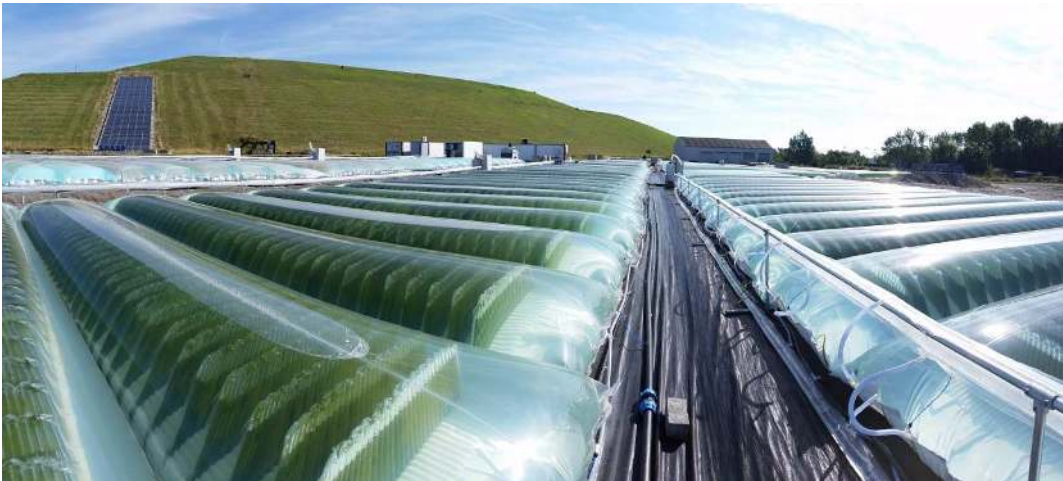
81 Fig 1: View of a ProviAPT™ microalgae production plant of 48 m 3 culture volume
