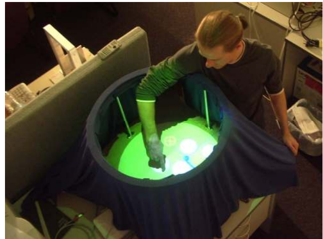
Figure 1 – An indoor user pointing at a location on the tabletop surface, which contains a virtual representation of the outdoor world. The table uses four video cameras to capture a 3D representation of objects located on the table.
