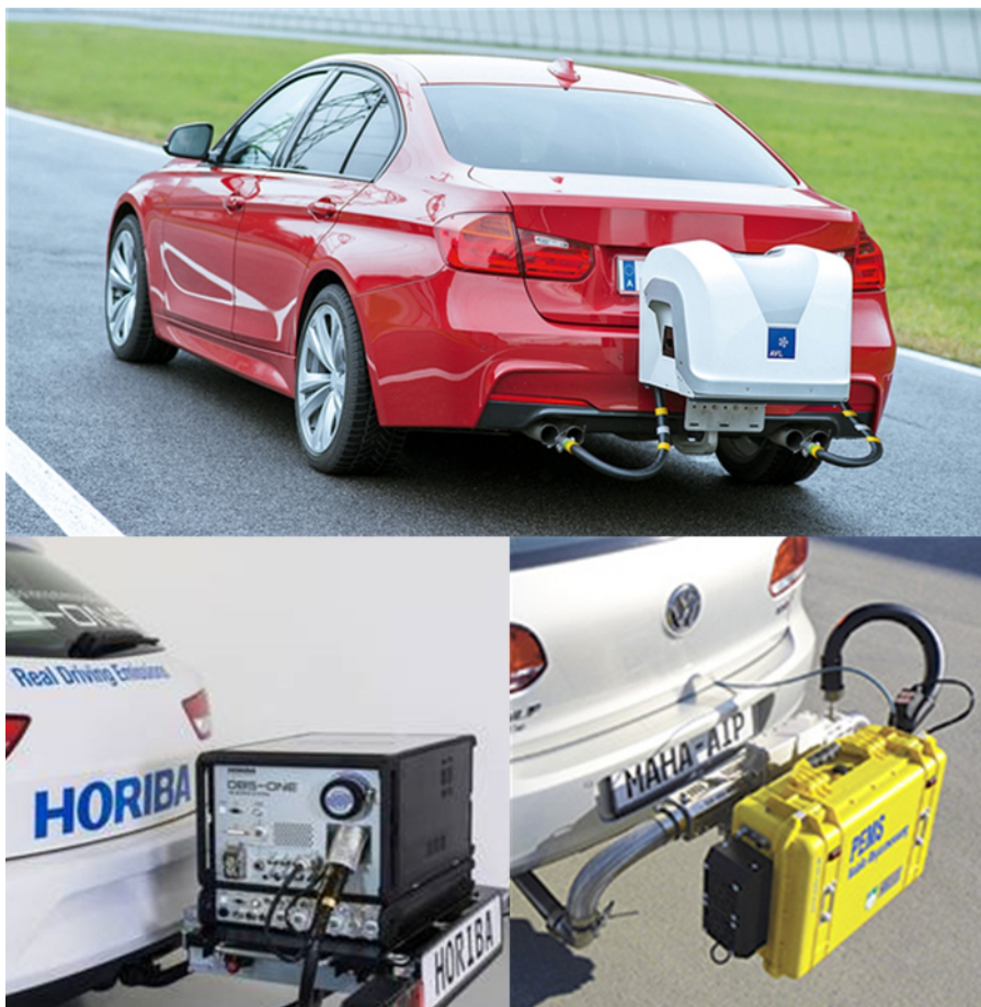
Figure 1: PEMS from different manufacturers. In these examples, the PEMS are installed outside of the vehicle on a support or on the tow bar. Please click here to view a larger version of this figure.
