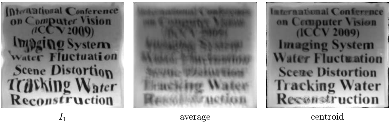
Figure 4: Result of the centroid method for the sequence from reference [21] (used with permission). This is a short sequence of 61 frames with rather large deformations, for which the average has not converged to a uniformly blurry image.
