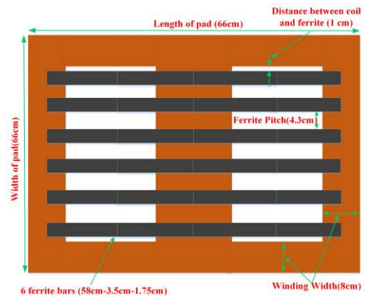
Fig. 12. Employed DD structure coil for 6.6 kW IPT charger
