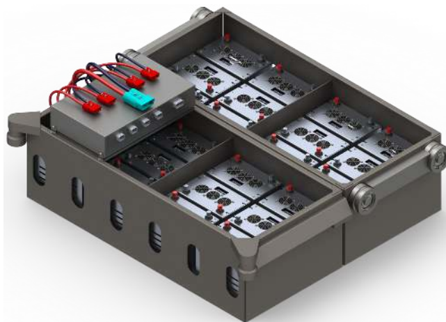
Fig. 7. 3D view of the redesigned battery of the minibus. Wiring harness is not shown.
