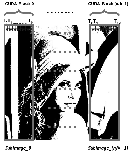
Figure 13: Mapping CUDA Blocks into subimages
