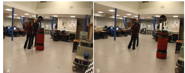
Fig. 6. A comparison between a classic motion planner and the human-aware navigation planner. Clearly the last one produces a more acceptable path by taking into account the safety and visibility of each human in the environment
