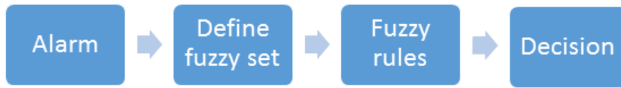
Figure 1: The method used for implementing fuzzy logics when developing intelligent alarms. The decision concludes whether the alarm is true or false positive.
