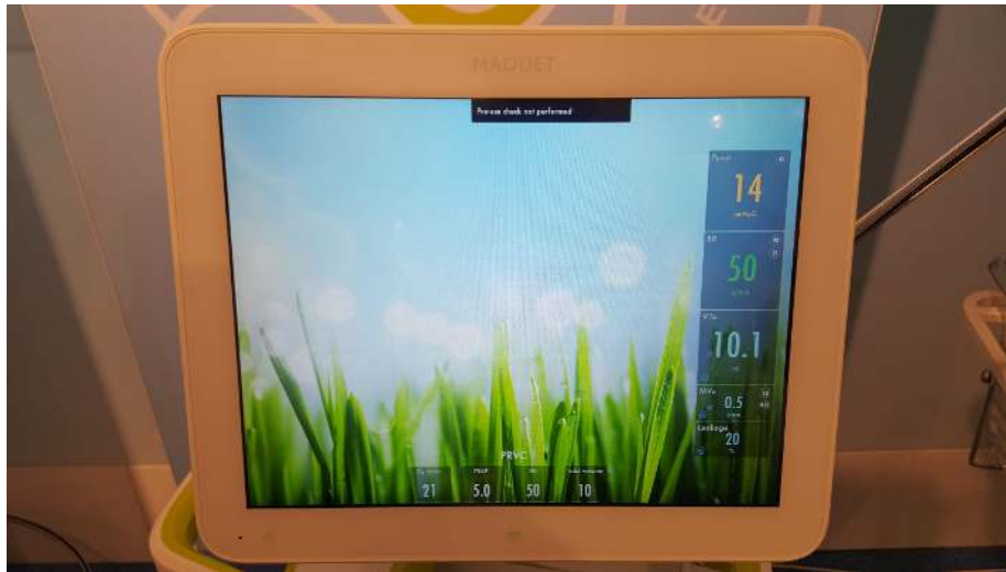
Figure B. 8 – The Family Mode in SERVOn ventilator from Maquet Critical Care.
