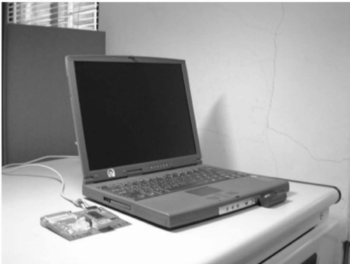
Fig. 10. AFS Bluetooth tracking prototype. (The notebook is the AP controller that connected to the VoIP system. The circuit board on the left of the notebook is the Bluetooth AP module.)
