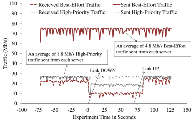
Fig. 6. Traffic for a client (client connected to Zagreb). Best-Effort Traffic is about 4.8 Mb/s and High-Priority traffic is about 1.8 Mb/s from each server
