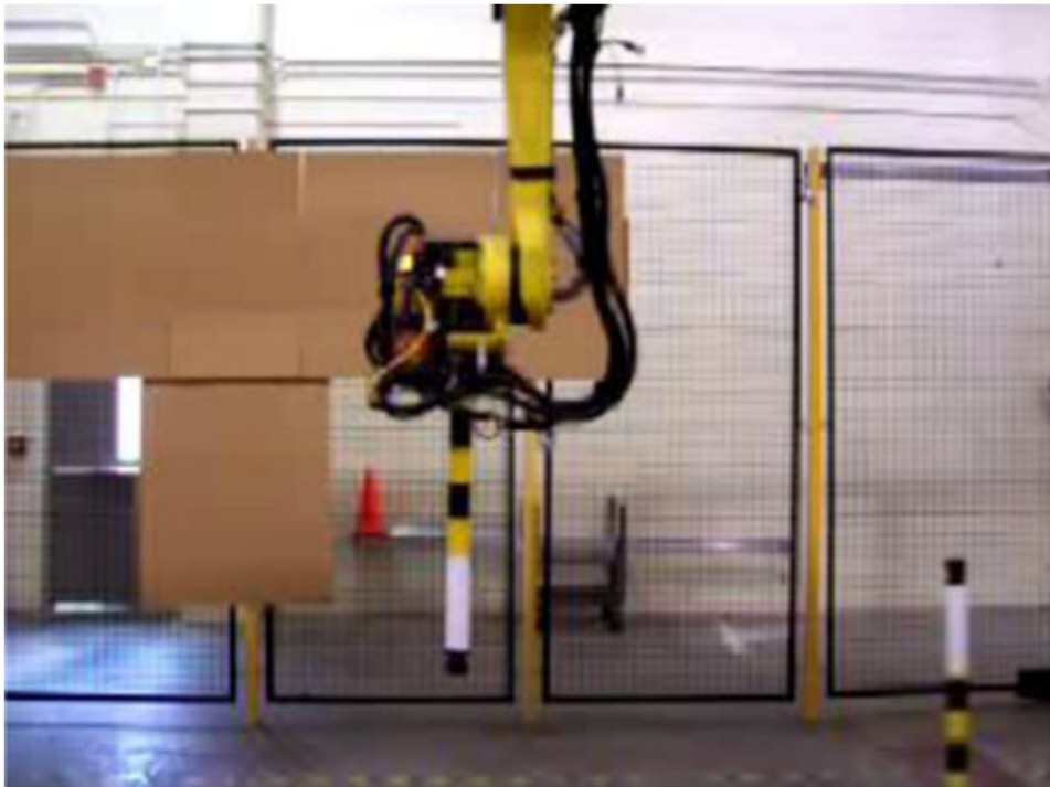
Fig. 9. Two retro-reflective targets, one representing a simulated human (right) and the other indicating the position of the robot (left) were tracked for SSM implementation testing.
