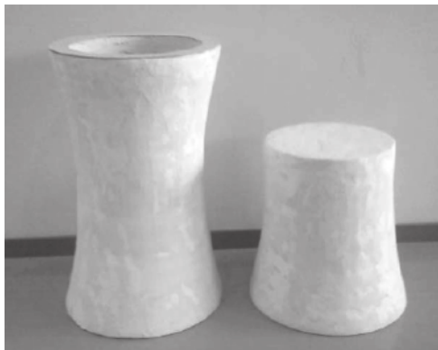
Figure 7-18 Foam prototype of the first splash design.
