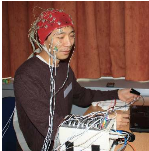
Figure 4.2: A participant wearing an EEG head cap with 32 electrodes. EOG and EMG flat electrodes are attached on the participant's face. The temperature, GSR sensors and plethysmograph are attached to the participant's left hand.
