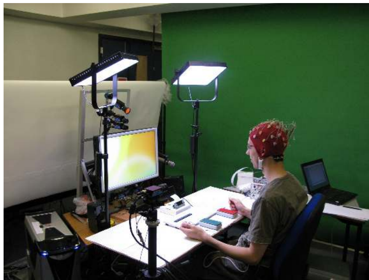
Figure 3.20: In the experimental setup, six video cameras were recording facial expressions. The modified keyboard is visible in front of the participant.
