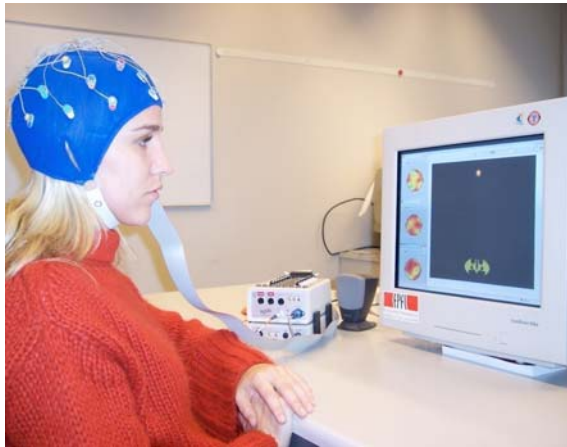
Figure 1. EEG signal acquisition setup.
