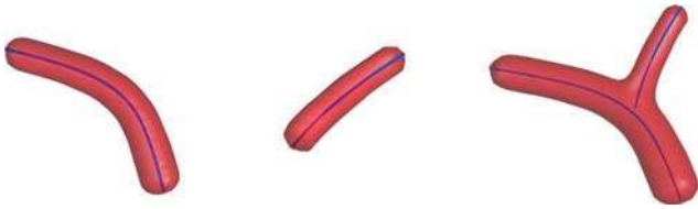
Fig. 5. Smooth blending of two implicitly defined shapes with \max_{n,\delta}(x, y) . Two individual implicit objects (left and middle) are smoothly blended as one implicit object (right) by using the smooth maximum function \max_{n,\delta}(x, y) .
